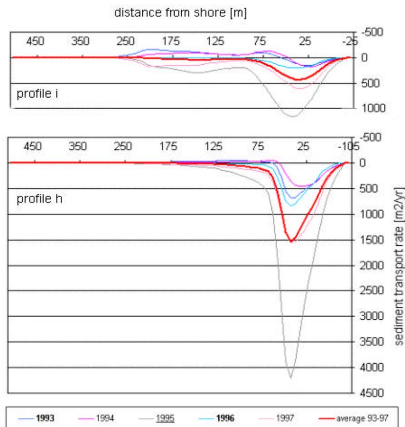
Figure 5: Sediment transport rates 1993–1997 at selected Hiddensee profiles (1D modeling)
