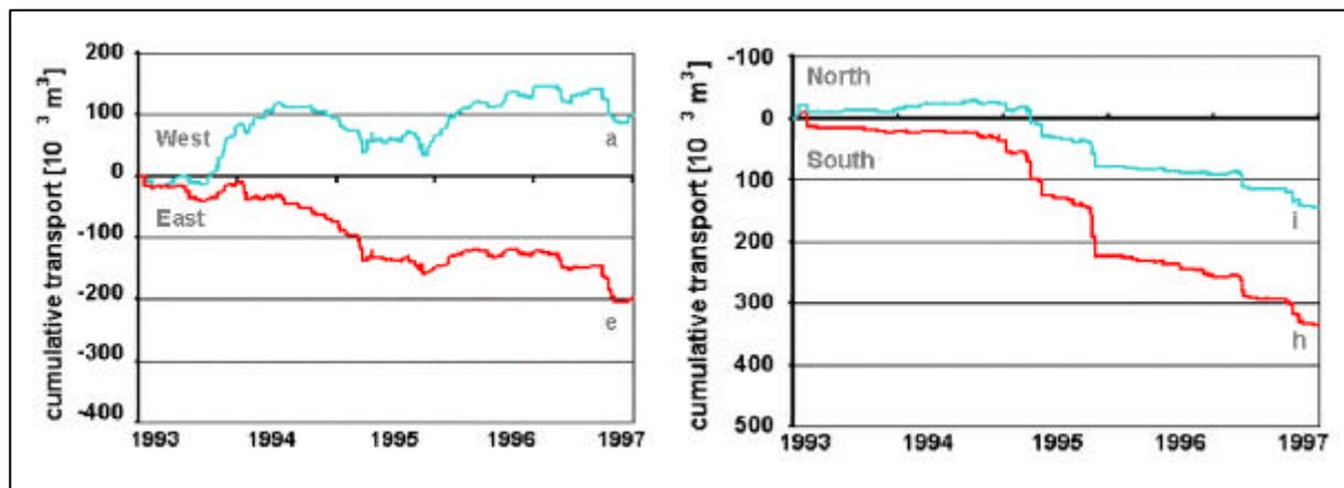
Figure 4: Cumulative sediment transport 1993 – 1997 (0D modeling)
