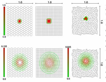
As initial condition a material concentration in the middle of the investigation area is injected. Figure 7 shows the used decompositions and the corresponding initial con-The ditions. used decompositions based on quadrangles and hexagons as well as on Voronoi cells.
