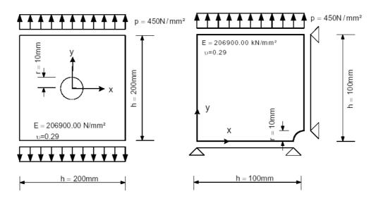
Figure 8: Structural system of the perforated pane
