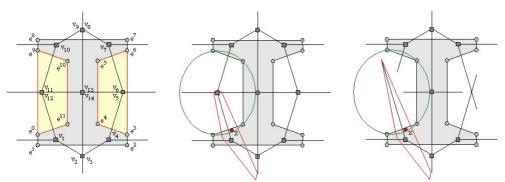
Figure 3: Voronoi decomposition of a non convex polyhedron
