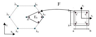
Figure 6: Transformation of the unit polyhedron to the convex polyhedron
